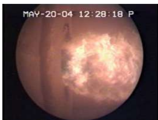
Figure 8. Experimental Furnace Flame Shape
